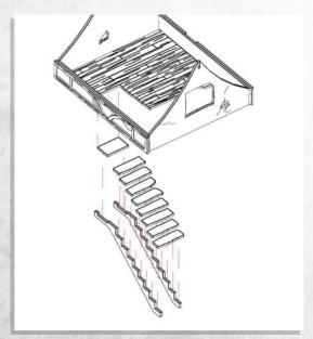
NOTE: Glue stairs to underside of floor where shown
