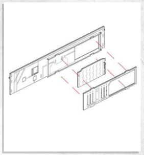
NOTE: Repeat for second door. NOTE: Place the door within the frame (DO NOT GLUE) to allow it to slide.
