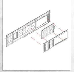
NOTE: Repeat for the second door. NOTE: Place the door within the frame (DO NOT GLUE) to allow it to slide.
