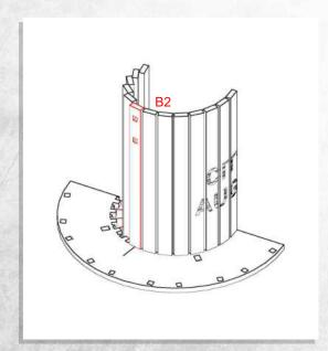
NOTE: Glue the red highlighted piece where the marking is.
