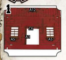
Glue 2x A5 together under each window (on part A12). Insert C6 then A3, making sure the notch at the bottom of A3 faces towards you.
