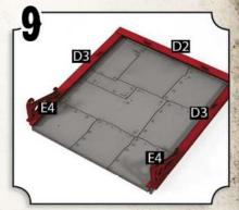
Connect each D3 to each A5, the corner notch on D3 should be facing outwards as shown.
